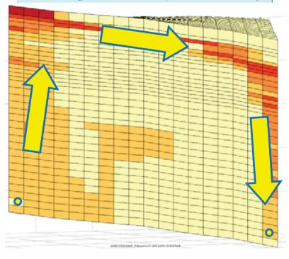
Moderate heterogeneity ( $V_{DP} \approx 0.6$ ) and moderate vertical permeability
